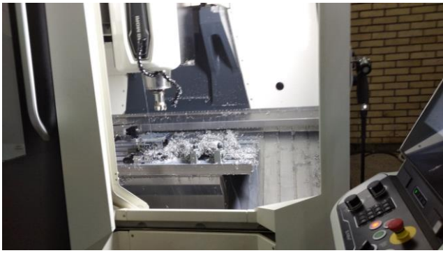
Fig. 8 Demonstration of CMX 600 V machining center operation (when machining gear pump cover)
