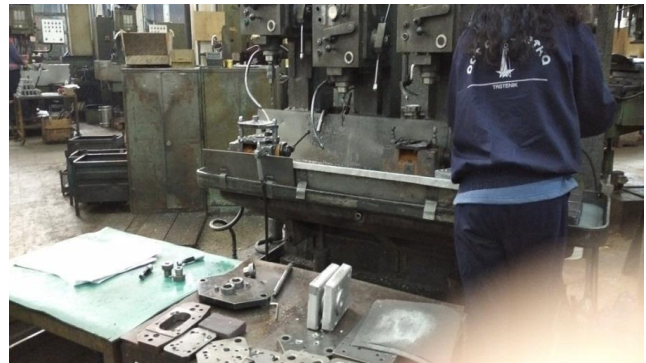
Figure 9. Appearance of the workplace where the drilling operation of the gear pump cover is performed
