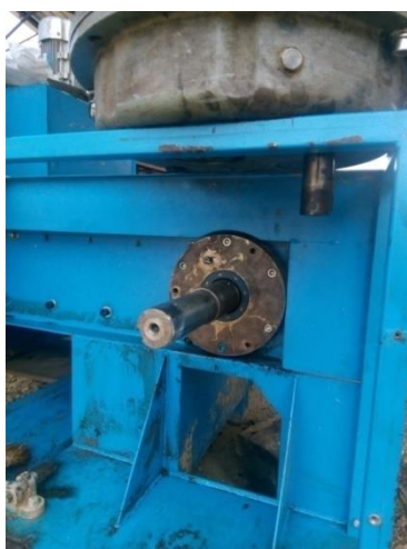
Figure 3. Layout of the attached roller on which the knives for chopping raspberry and blackberry cuttings
